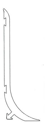
Easycove® cove base moldings, pre-formed with a patented watertight design, specifically geared for the floor and wall coatings industry.
